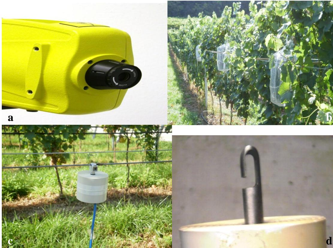
**Figure 2.** Laser vibrometer (a) and field test overview (b): net sleeves were mounted around grapevine shoots at different distances from the shakers. The first model of shaker (2011, c) was fixed with a screwdriver to the wire; the second model (2012, d) was hung with a special hook.
